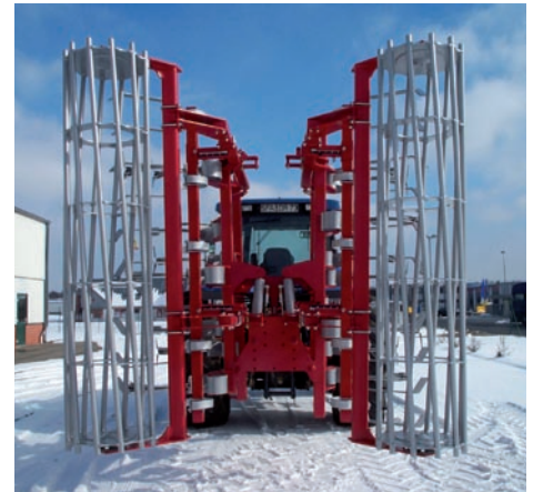
Vibro Flex 7400 folded in transport position.
